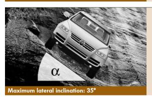
The steepest slope a vehicle can drive laterally. The Touareg will comfortably function to a slope up to 35 degrees.
